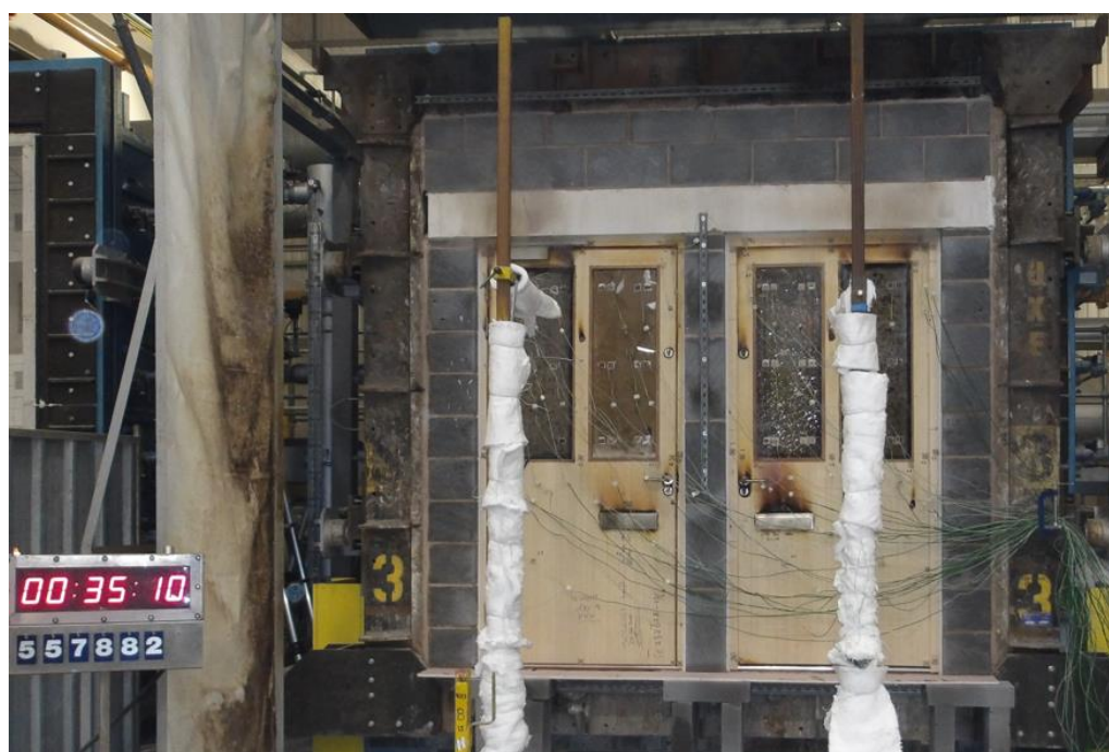
The unexposed face of the doorsets after a test duration of 35 minutes
