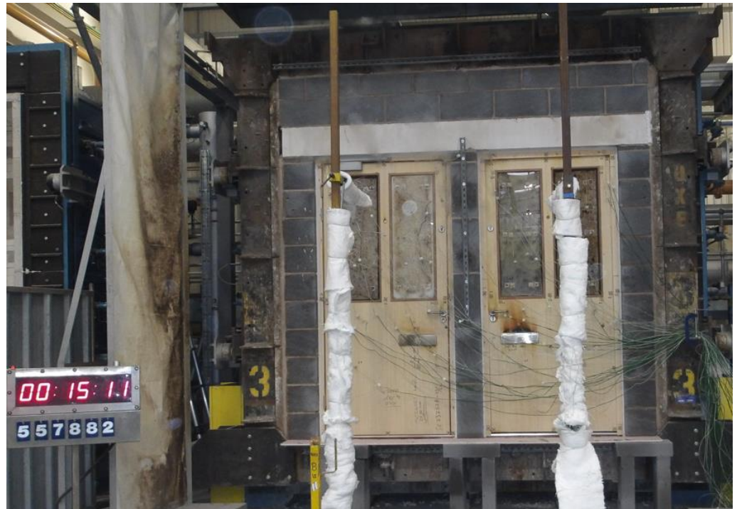
The unexposed face of the doorsets after a test duration of 15 minutes
