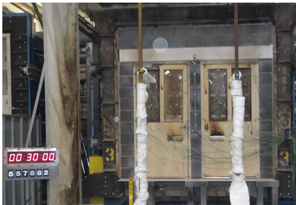
The unexposed face of the doorsets after a test duration of 30 minutes
