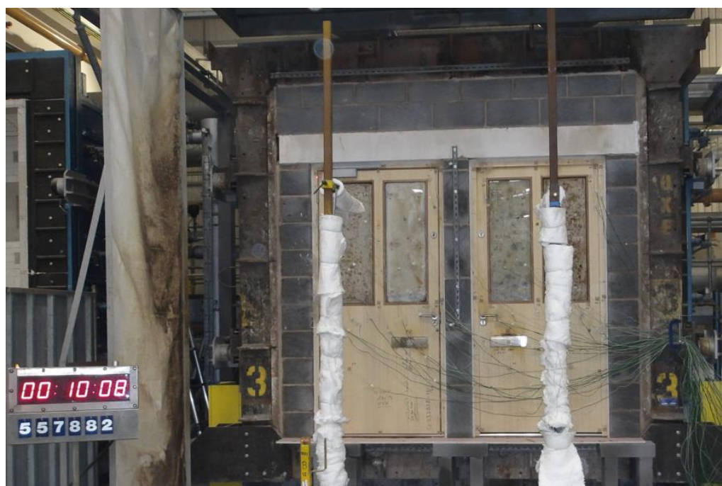
The unexposed face of the doorsets after a test duration of 10 minutes
