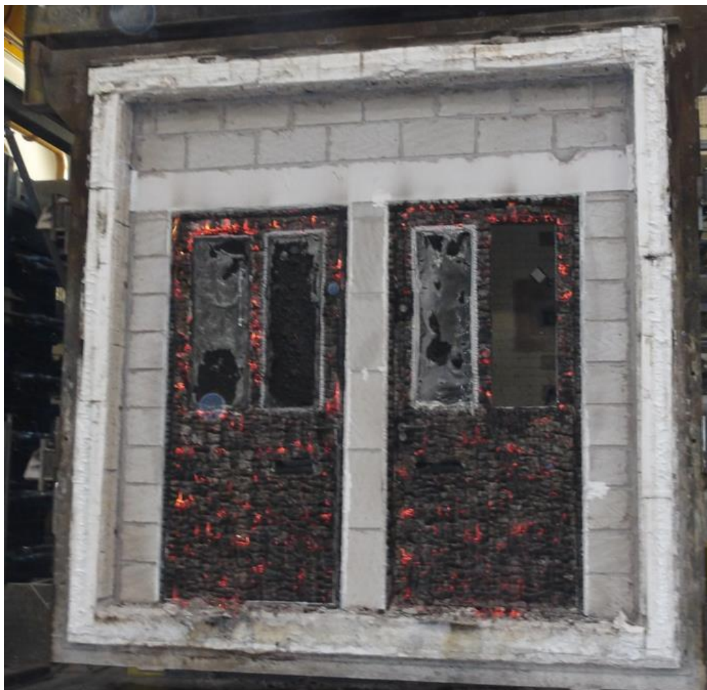
The exposed face of the doorsets immediately after the test
