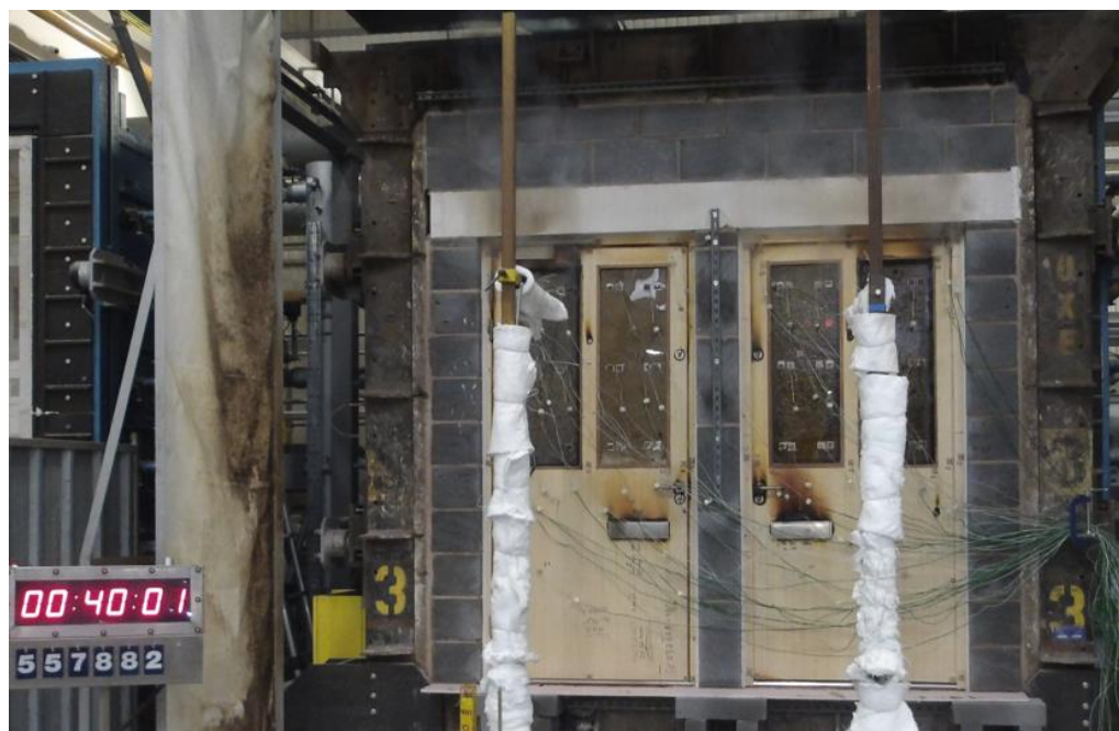
The unexposed face of the doorsets after a test duration of 40 minutes
