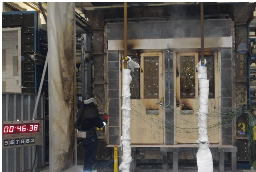
The unexposed face of the doorsets after a test duration of 46 minutes showing sustained flaming on Doorset A
