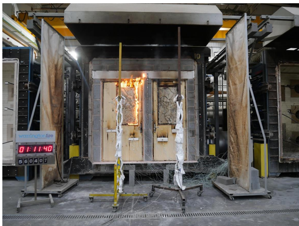
The unexposed face of the specimen after a test duration of 71 minutes
